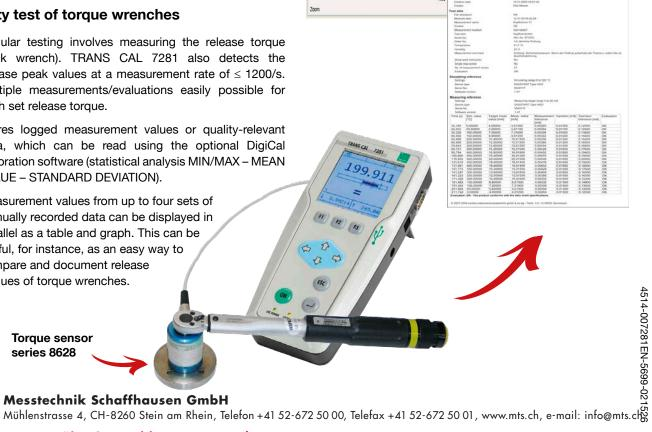
The high-precision calibrator and tester model 7281 is ideal for locating faults in measurement systems. For display devices based on strain gauge sensors, the stored characteristics values can be simulated in an infinitely adjustable range of  $\pm$  3 mV/V and  $\pm$  50 mV/V. In this case it is also important to measure the excitation voltage for strain gauge sensor in order to rule out any problems here.
