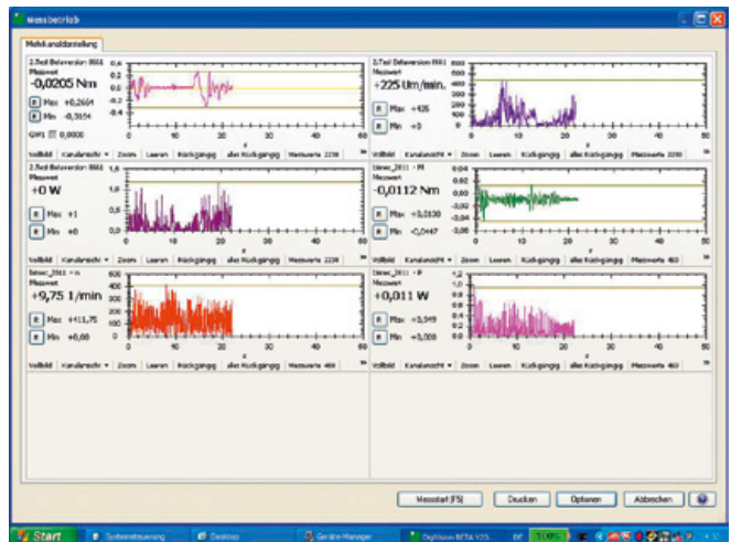
Screenshot P100: Multichannel display of two sensors, torque / speed / mechanical power
