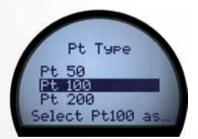
PR's well-known user-friendly menu structure provides a guided configuration path that makes setting up the transmitter fast and intuitive.
