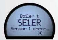
If a sensor or device error occurs, a red or white flashing backlight, specific error text, and scrolling error messages help you provide quick troubleshooting.
