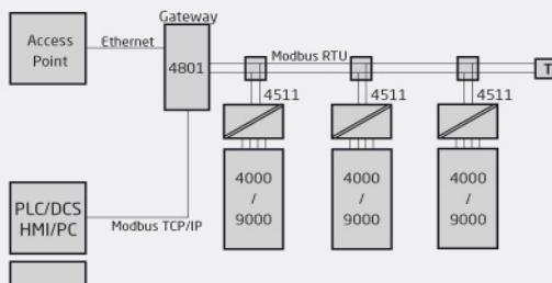
Up to 32 devices per segment without the use of a network repeater
