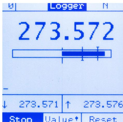
5. Press the **[F2]** key to record measured values manually. The number of measured values that have been recorded is shown in the function field for the **[F2]** key.
