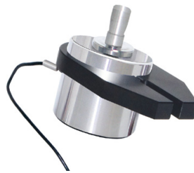
Mounting the catch on the load cell
