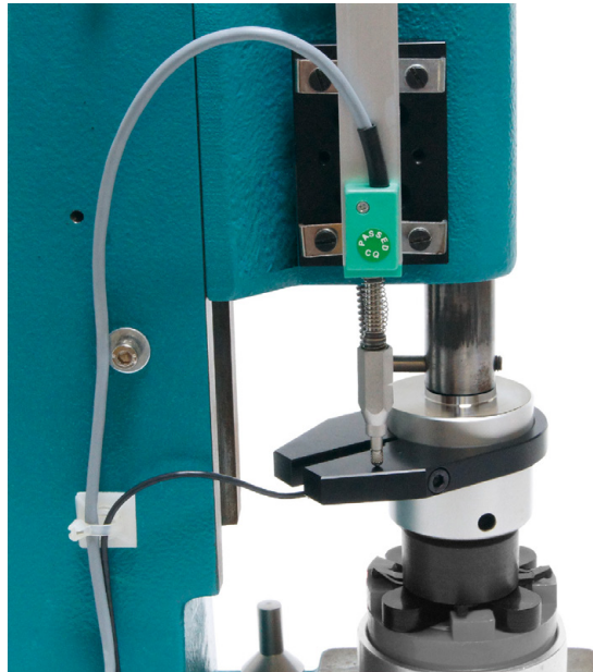
Displacement measurement system (DMS) in the lower position
