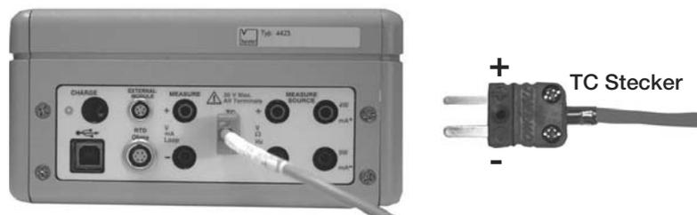
Figure 7: Measuring Temperature Using Thermocouple Terminals
