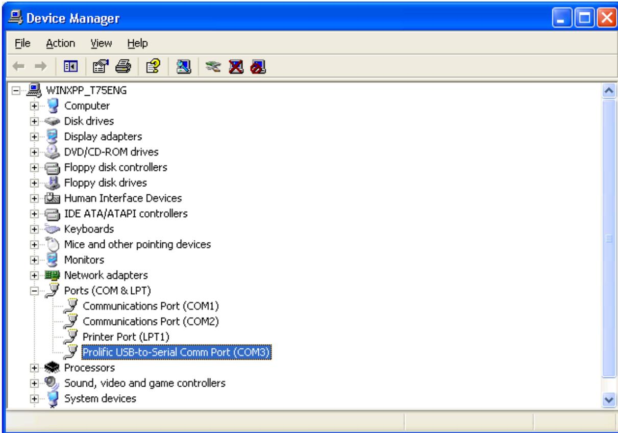
You'll find the calibrator at the entry "Prolific USB-to-Serial COM Port". Beyond this entry you'll see the assigned COM-port. You have to set up this COM-port at the software; you use to communicate with the calibrator.
