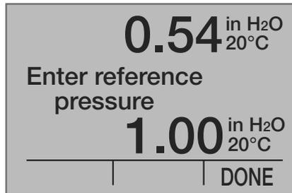
The value displayed on the top line is the current pressure reading adjusted with the current reference pressure.
