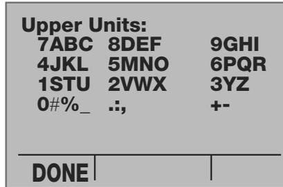
Up to 5 characters may be entered for a unit description using a mobile phone style entry method. The four lower lines provide a mapping of the allowed alphanumeric characters to the numeric keypad keys.
