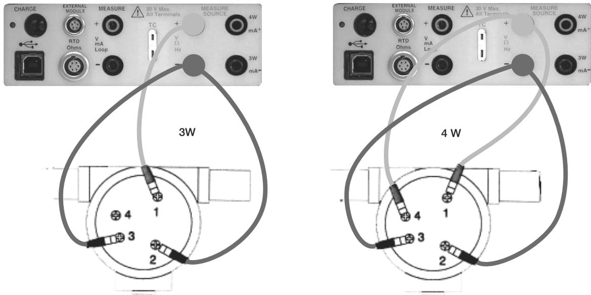
Figure 15: Using a 3- or 4-wire Connection for RTDs
