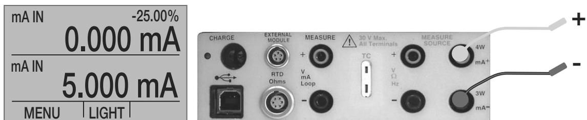
Figure 6. Measuring mA with Input/Output Terminals
