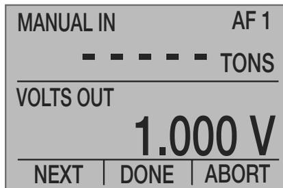
The current test type, “AF” for As Found, and point number are shown in the upper right corner of the display.
