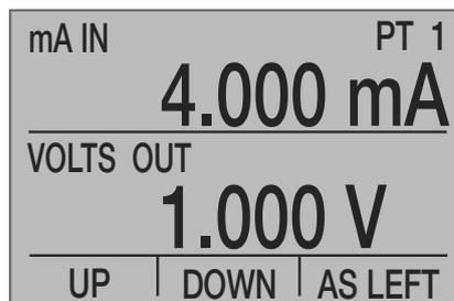
The "PT" in the upper right corner of the display indicates that this is the adjustment display. If an As Found data point is being generated, its number is displayed. If a user-entered value is being generated, two dashes are displayed.
