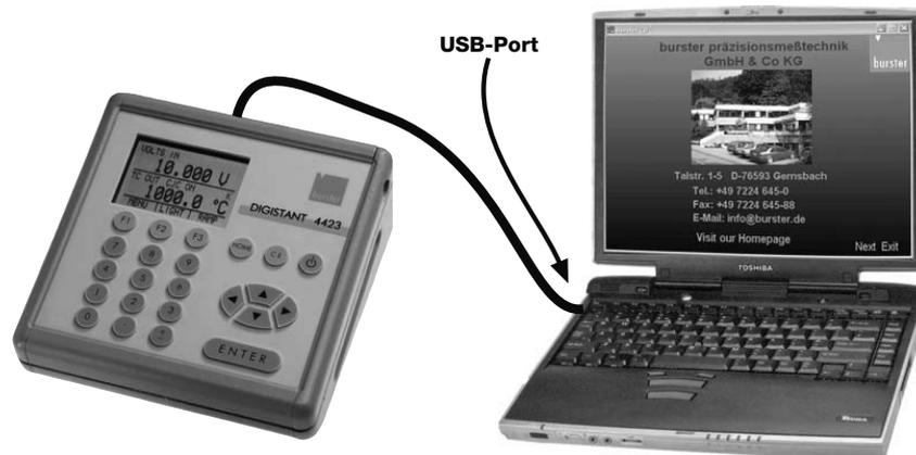
Figure 23: Calibrator-to-Computer Connection
