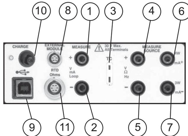
Figure 1. Input/Output Terminals
