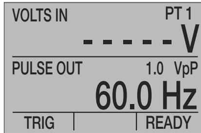
The “PT” in the upper right corner of the display indicates that this is the adjustment display. If an As Found data point is selected, its number is displayed. If a user-entered value is selected, two dashes are displayed.
