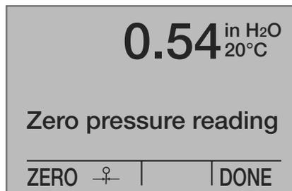
The value displayed on the top line is the current pressure reading adjusted with the current zero value.
