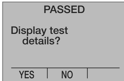
The overall test status is displayed on the top line. If all points passed, "PASSED" is displayed. If one or more points have failed, "FAILED" is displayed.
