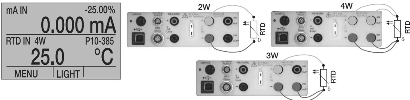
Figure 8. Measuring Temperature with RTD Connection
