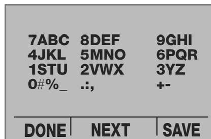
Up to 16 characters may be entered for the field using a mobile phone style entry method. The four lower lines provide a mapping of the allowed characters to the numeric keypad.
